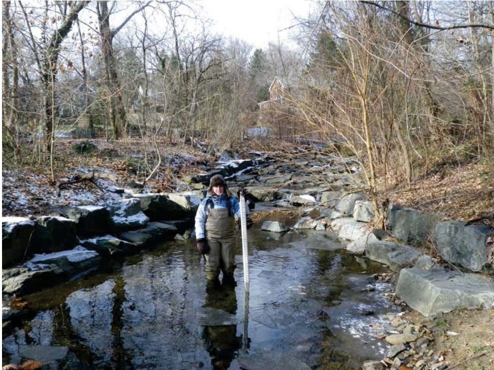
Photo 8. Middle Stony Run. Cross vane 14 at station 25+40 showing shallow pool.
